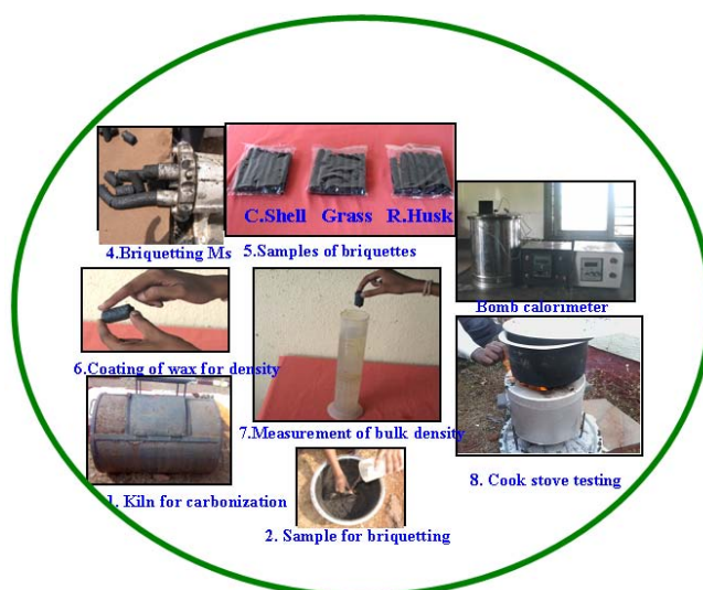
Figure 1 : Complete setup for briquettes preparation and testing
