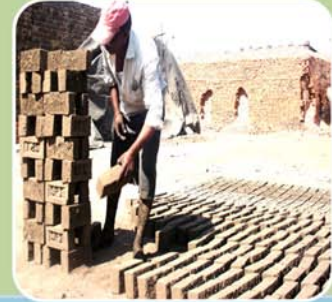
Bricks are kept as these structures to aerate all surfaces equally. for 2 days
