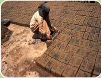
On an average a worker moulds about 1500 bricks in a day. The batch is dried in open for 3 days in the same position.
