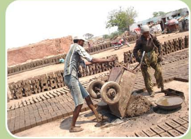
A worker is assigned the job of moulding clay into bricks
