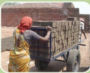
The bricks are carried to the kiln for heating process in a trolley (hand pulled). It carries 250 bricks at once.
