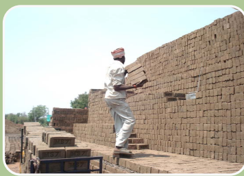
The batch of bricks is arranged as a heating hub
