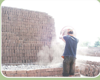
Another layer of coal is spread on the 6th brick mat.
