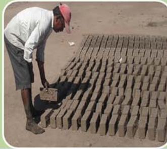
Bricks ' position is changed to dry the beneath area for 2 days
