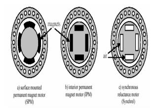
Figure 2 : Cross section of the three main types of PMSM
