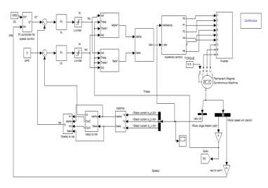
Figure 11 : Simulation circuit of PMSM Drive circuit
