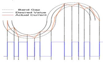
Figure 10 : PWM signal from Hysteresis controller
