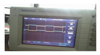
Figure 16 : gating signal showing delay
