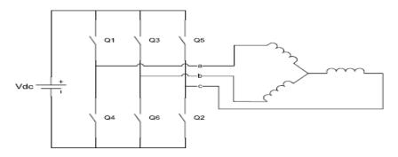
Figure 6 : Voltage Source Inverter Connected to a Motor
