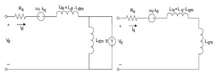
*Figure 5* : Equivalent circuit of Permanent Magnet Synchronous Motor
