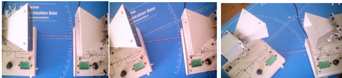
Figure 7 : Original Photographs of Move the Receiver around the Transmitter on the Semi-Circular Line
