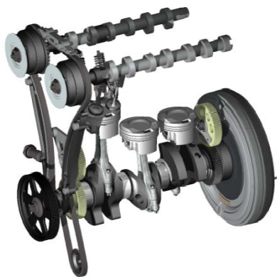
Figure 1 : Functional layout diagram of crankshaft
