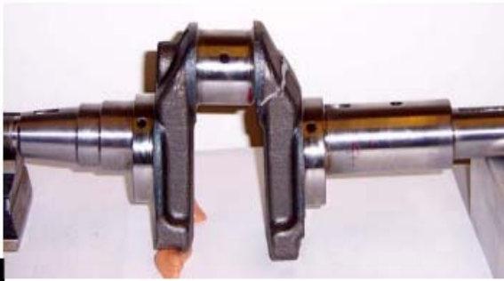
Figure 3 : Failure occurred area of crankshaft (i)
