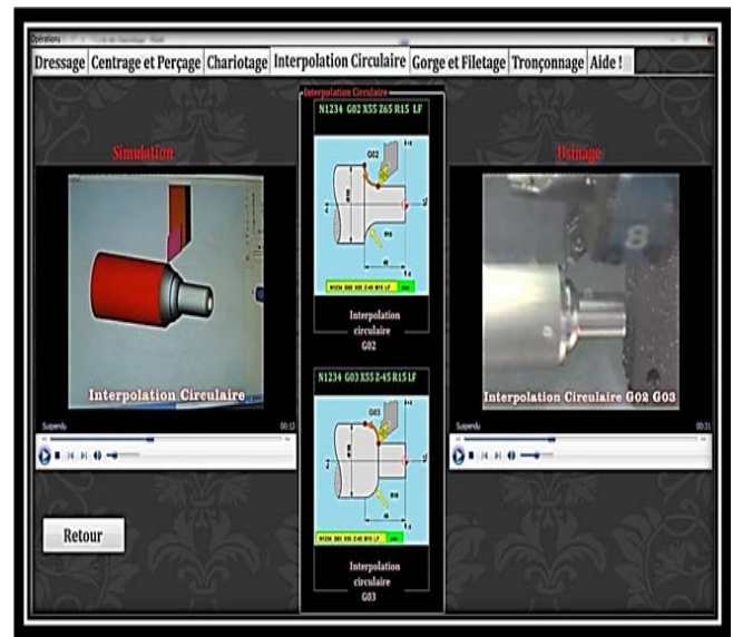
Figure 5 : Example of circular interpolation in turning
