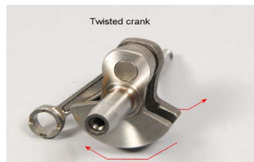
Figure 7 : Side view of crankshaft showing changes in its lob shape
