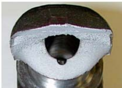
Figure 4 : Failure occurred area of crankshaft (ii)
