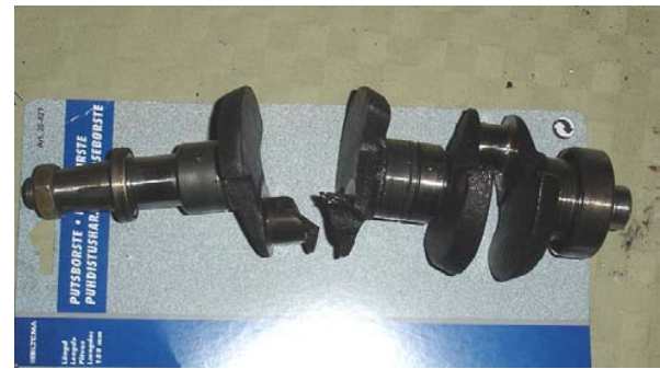
Figure 5 : Final stage of failure occurred in the crankshaft (iii)
