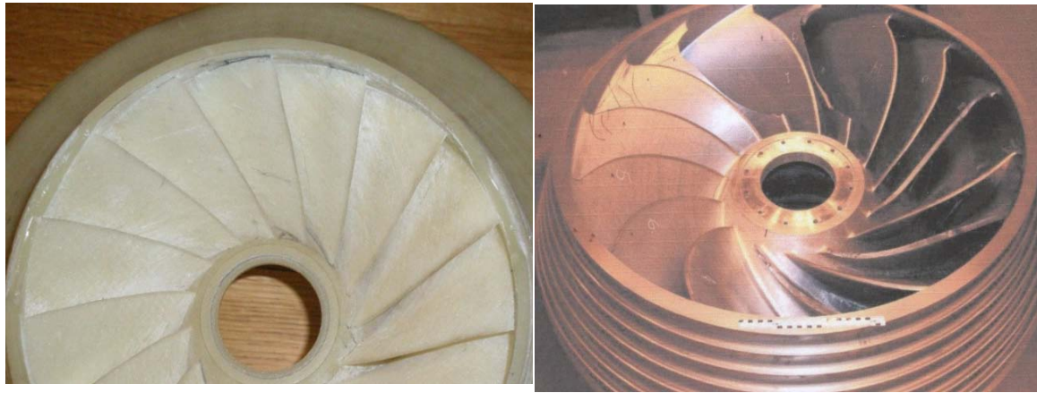
Figure 10 : Traditional Kvaerner runner (Lu Buge Power plant in CHINA) with skewed relative straight blade outlets (left) compared with the blade outlets of Sunnå Høy, where the cracked blades are shown. After repair and cutting the blade outlet edges straight no further cracking was observed
