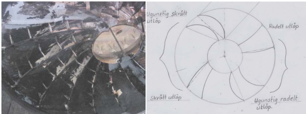
Figure 9 : LEFT: The outlet of the high head Francis turbine runner at Ste-Marguerite (SM3) in Canada. Note the reinforcements between the curved blade outlet for temporary operation of the runner. (Described in /Ref. 4/) RIGHT: Curved and straight radial blades outlets (right side)-and curved and straight skewed blade outlets (left side)
