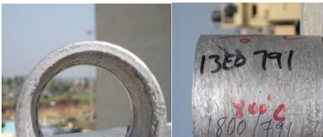
Figure 2 : Castings of 8 mm-thick cylinders
