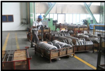
Figure : Excessive push and pull while transportation between stations
