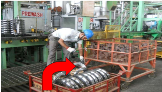
Figure : Excessive Bending on crown Wheel
