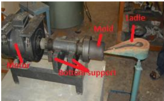
Figure 1 : Centrifugal casting set up
