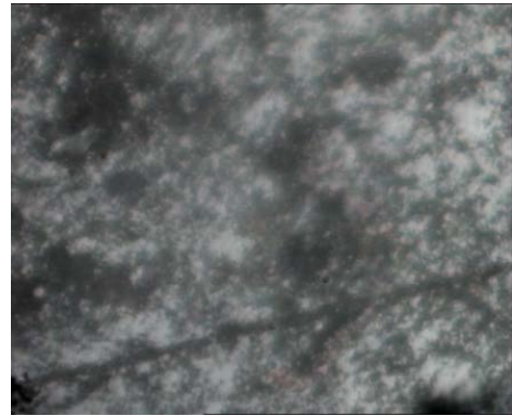
Figure 1 : Image of cutting tool before cryogenic treatment (magnification X600)
