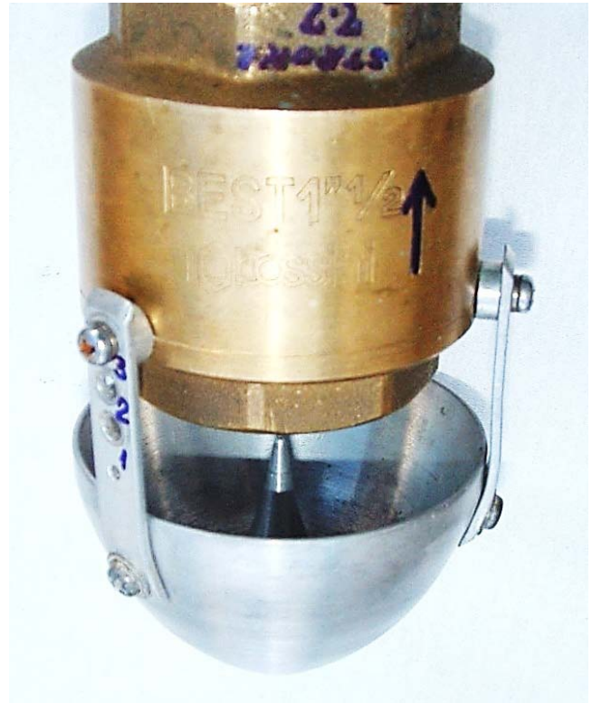
Figure 3 : Assembly view of the parabolic deflector as connected to the 1.5" spring-loaded poppet valve, No. 3
