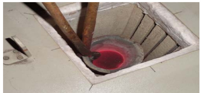
Figure 2.3 : Preheded Mixer of SiC and Graphite Powder
