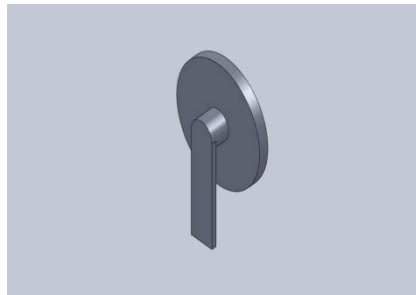
Figure 3(c) : Disc of a universal coupling
