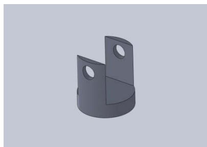
Figure 3(a) : Yoke of a universal coupling
