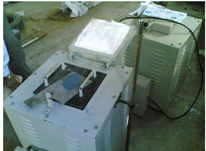
Figure 2.1 : Muffle Furnace used for Fabrication of Hybrid Composite
