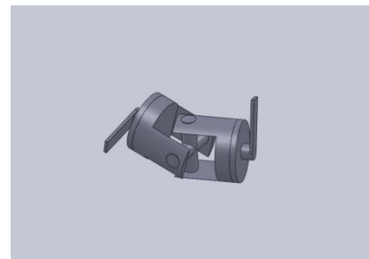
Figure 2 : CAD design of a universal coupling
