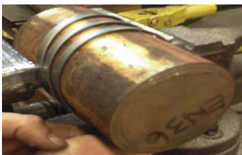
Figure 2 : Experimental simulation of reverse bending of wires for civil engineering applications
