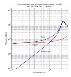
Figure 3: Attenuation of oxygen and water vapor (density 7.5 g/m³) for horizontal path (1-30GHz)
