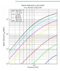
Figure 6: Specific attenuation due to rain for an elevation angle of 90°
