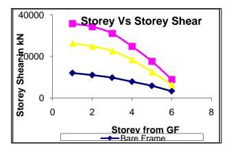
Figure 5: Story Level from Ground Floor Vs Story Shear
