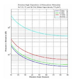
Figure 4: Elevation angle dependance of atmospheric attenuation for 3,6,12 & 24GHz(water vapor density 7.5 g/m³)
