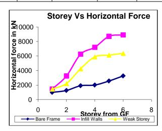
Figure 3: Story level Vs Horizontal Force Curve
