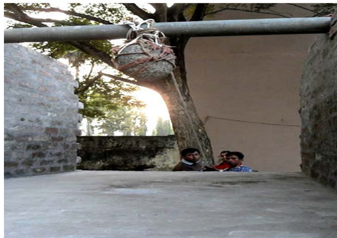
Figure 11 : Impact test setup with round hammer ball, 1m free fall on slab
