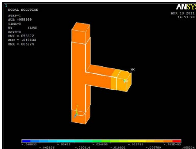
Displacement Solution For Beam-Column Joints As Per Code IS 456 Retrofitted Specimen 66.9 kN
