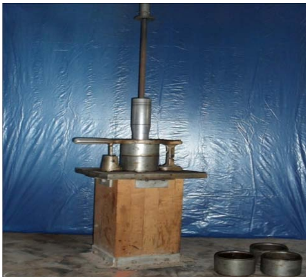
Figure 1 : Photographic views of pedestal hammer and mould used in preparing Marshall Test Specimen
