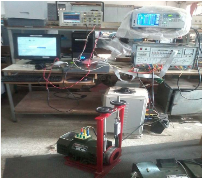
Figure 3 : Experimental Setup of Indirect Vector control with stator resistance estimation
