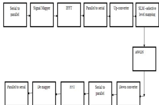
Figure 2.1 : Block diagram of an OFDM system
