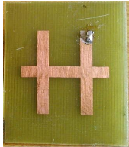
Figure 17 : Hardware of Proposed MSA
