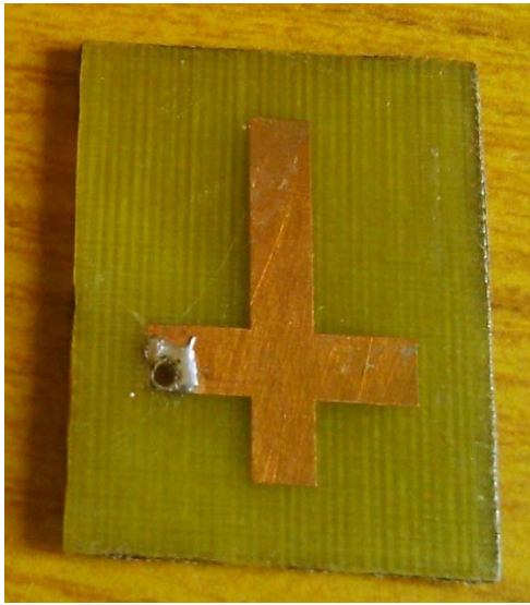
Figure 12 : Hardware of Proposed MSA
