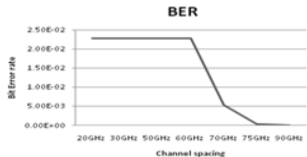
Fig.17 : BER factor Vs channel spacing
