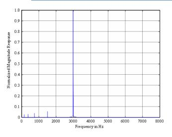
*Figure 6 :* Responses from five sinusoids. Their amplitudes were originally equal but now reflect the effects of gain
