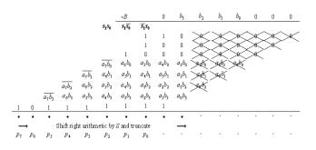
Figure 2 (b): Multiplication with coefficient shifting. S = 3
