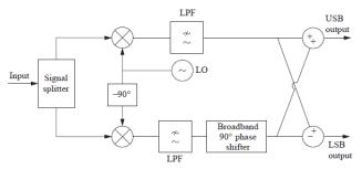
*Figure 4 :* The arrangement of an image reject mixer, translating the input signal (centered on the same frequency as the local oscillator) to centered on 0 Hz. Where the signal and local oscillator frequencies differ, giving a finite intermediate frequency, the low-pass filters would be replaced by band-pass filters
