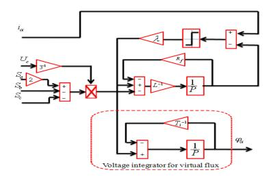
Figure 3 : Sliding-mode current observer for virtual grid flux
