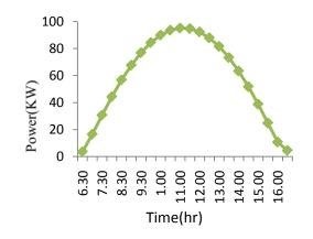
*Figure 11 :* Power data obtained against Time when Tilt/Azimuth is 1<sup>0</sup>/0<sup>0</sup>
