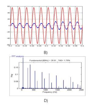
Fig.7. Simulated responses for a step change in the load resistor: A) Harmonic currents injected by the active power filter, Load change at 0.3 s. B) Source voltage, source current. C) DC side capacitor voltage and filter D) Current spectrum harmonic: Grid in Phase 1.
