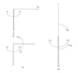
*Figure 5 (a)*: Showing how, for a positive frequency *f*s, the Q channel baseband output leads the I channel by  $90^{\circ}(b)$  After a  $90^{\circ}$  phase shift, the components due to +fs in both channels are in phase, those due to -fs in anti phase. So summing recovers the upper sideband; differencing, the lower
