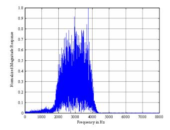
*Figure 8 :* Response of each filter with its associated gain from a white noise input
