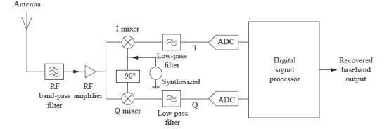
Figure 7 : Block diagram of a digital receiver, using an image reject mixer followed by digital signal processing
