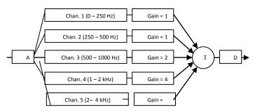
*Figure 4 :* Block diagram of digital signal processing Stage
