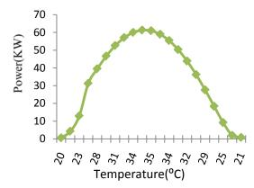
*Figure 6*: Power data obtained against Temperature when Tilt/Azimuth is 21<sup>0</sup>/180<sup>0</sup>
