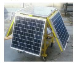
*Figure 3 :* Orientation of PV modules at 4 different slopes [9]
