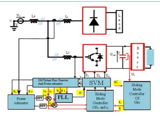
Figure 1 : Scheme of the multi-function converter
