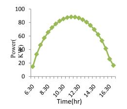
Figure 12 : Power data obtained against Time when Tilt/Azimuth is  $90^{0}/0^{0}$
