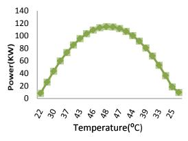
*Figure 5*: Power data obtained against Temperature when Tilt/Azimuth is 21<sup>0</sup>/0<sup>0</sup>
