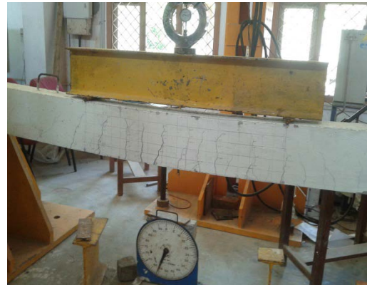
Figure 6 : Crack Pattern GPC-I Beam
