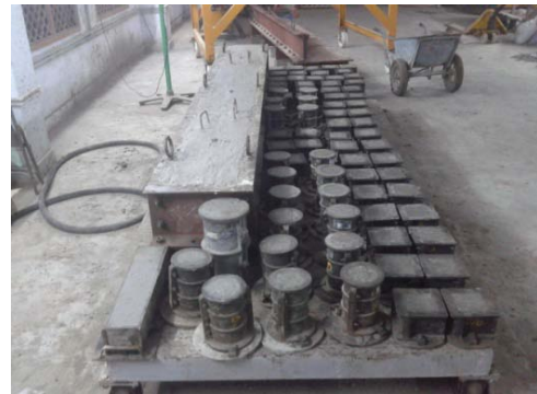
Figure 3 : Casting of Specimens
