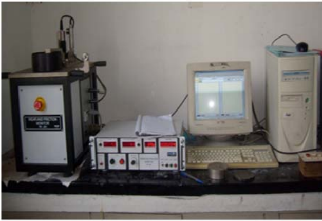
Figure 5 : Pin on disc experimental setup
