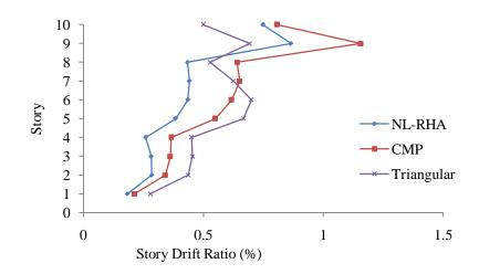
Figure 4.2: Height-wise distribution of drift ratio for asymmetric model with 10% eccentricity
