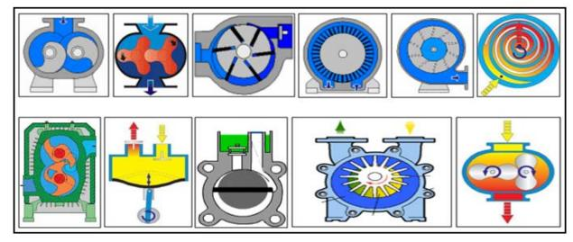
Figure 4. Schematic of working principle of some positive displacement pumps [6]
