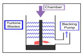
*Figure 7*: Schematic of Turbo-molecular Pump working principle
