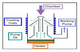
*Figure 6 :* Schematic of Diffusion Pump working principle
