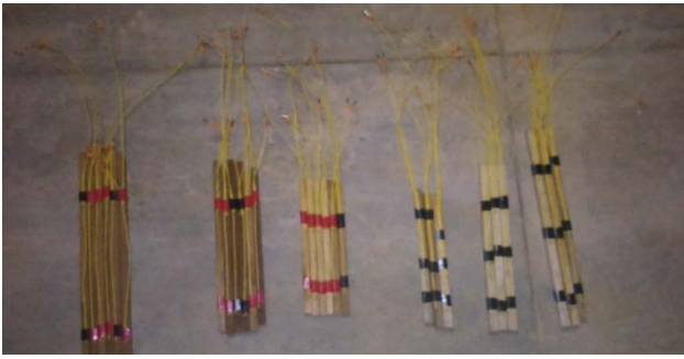
Figure 2 : Fixing of Thermocouple on wooden beads
