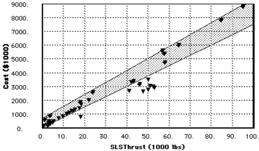
Figure 2 : Engine prices (\$1990) vs. SLS thrust (lbs)
