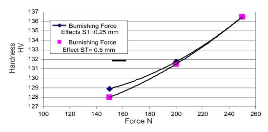
Figure 5: (b) The effect of burnishing force on the Surface Hardness under high table speed
