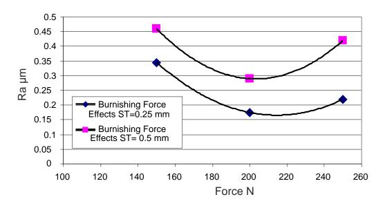
Figure 4: (a) The effect of burnishing force on the surface roughness under low table speed (=40 mm/min)
