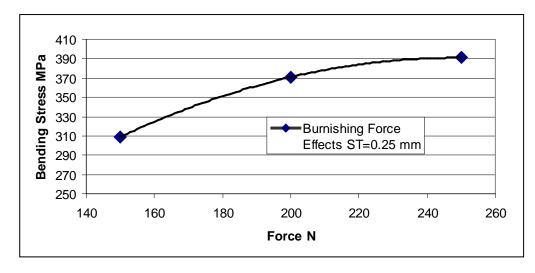
Figure 6: The effect of burnishing force on the bending stress
