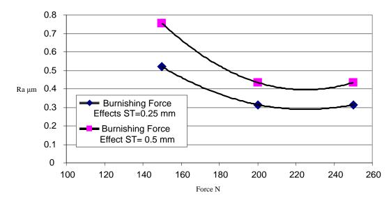
Figure 4 : (b) The effect of burnishing force on the surface roughness under high table speed (=120 mm/min)
