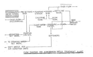
Raw water pumped from the lake to underground water storage tank Depth 8,0 m ,water stays for about one hour then water is pumped to the coagulation & settling tanks .
