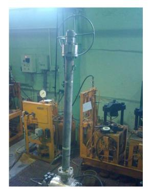
*Figure 4 :* Drive of the ball valve DU-160 with extension column
