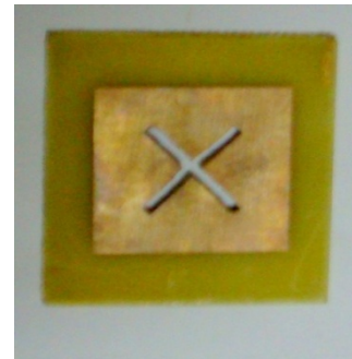
Figure 2.3 : RMSA with X-slot (on first substrate)
