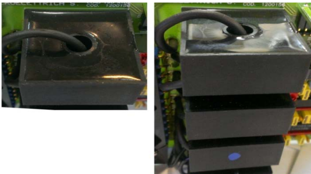
Fig. 3 : Encapsulated current transformers with epoxy capsulated secondary winding hardened in vacuum. You can clearly see the primary winding, which consists of a single coil of flexible insulated wire
