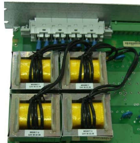
Fig. 2 : Example of a module of analogue inputs of DPR with installed CT. You can clearly see the primary winding, which consists of 4 coils of flexible insulated black wire
