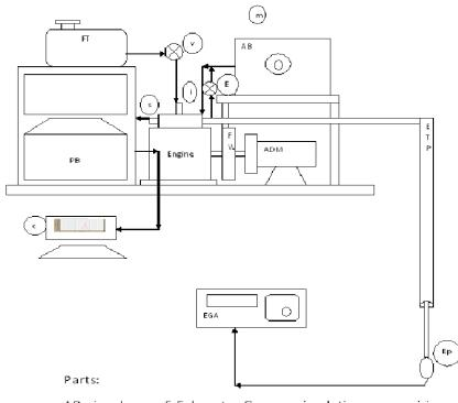
AB-air box ,E-Exhaust Gas recirculation perocision,mmeasurement of air by mano meter , Fw-fly wheel, ADMalternator dynamometer, i-fuel injector,C-computer for P- $\theta$
