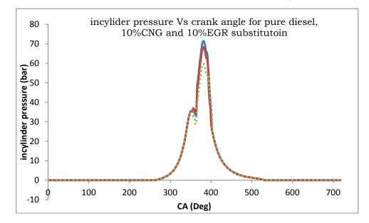
Chart 8 : in-cylinder pressure Vs crank angle for pure diesel, 10%CNG and 10%EGR substitution
