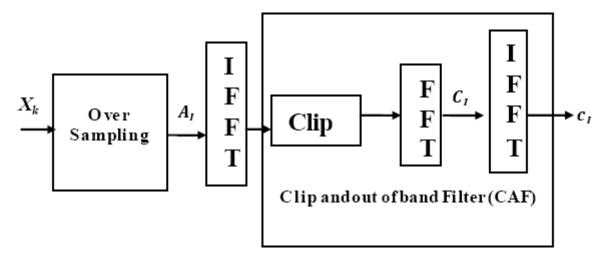
Fig 3: Repeating clipping and filtering technique
