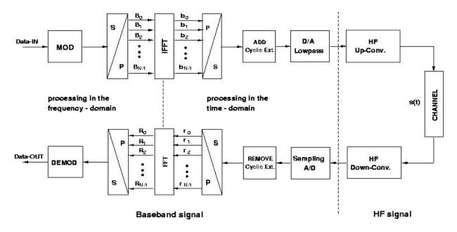
Fig 1: OFDM system model
