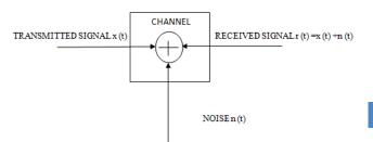
Figure 4: Block diagram of AWGN channel
