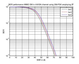
*Figure 5*: (h) BER performance of MIMO SM using 256-PSK in AWGN channel
