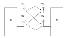
*Figure 1 :* MIMO system with 2 transmit and 2 receive antennas
