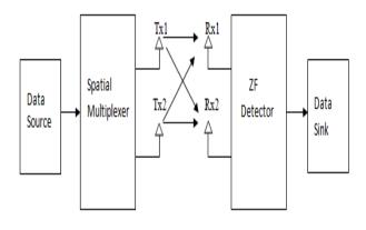
Figure 2: MIMO Spatial Multiplexing system
