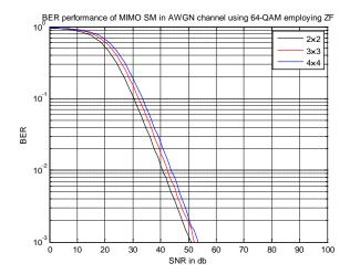
*Figure 6 :* (c) BER performance of MIMO SM using 64-QAM in AWGN channel
