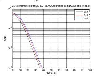
Figure 5(a)-(j) BER vs. SNR plots over AWGN
