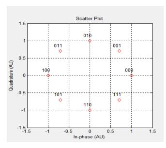
Figure 3 : Signal space for 8-PSK
