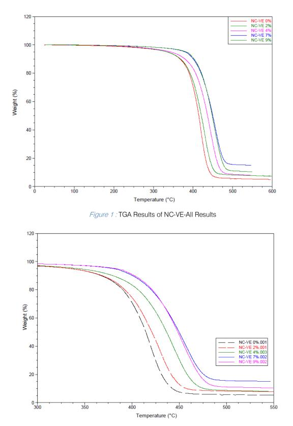
Figure 2 : TGA Results of NC-VE-All Results with Zoom at the Decomposition Region
