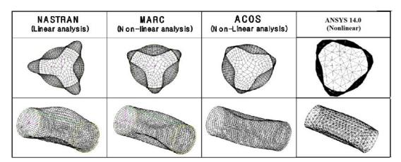
*Figure 5 :* Buckling modes of the [±45/90] FW composite cylinder *Table 1 :* Experimental And Finite Element Buckling Pressure (Unit: Mpa)
