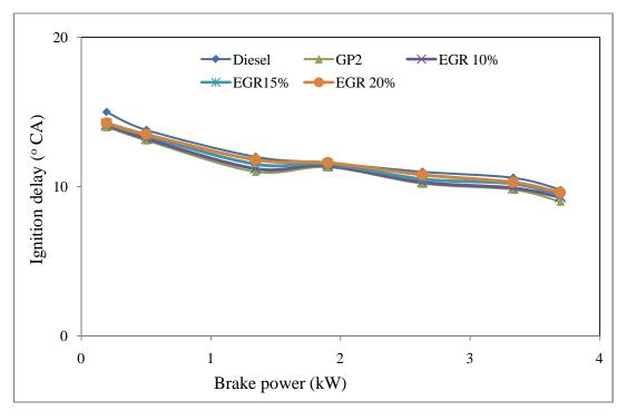
Figure 4 : Comparison of Ignition delay with different percentages of EGR
