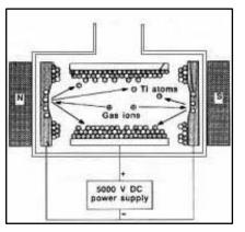
*Figure 8 :* Schematic oflon Pump working principle
