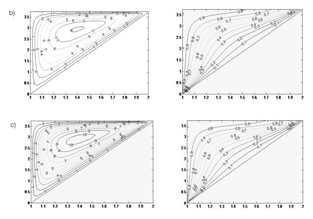
Figure 4 : Streamlines (left) and Isotherms (Right) for  $\epsilon$ =0.003, C<sub>A</sub> =15, R<sub>r</sub>=1
