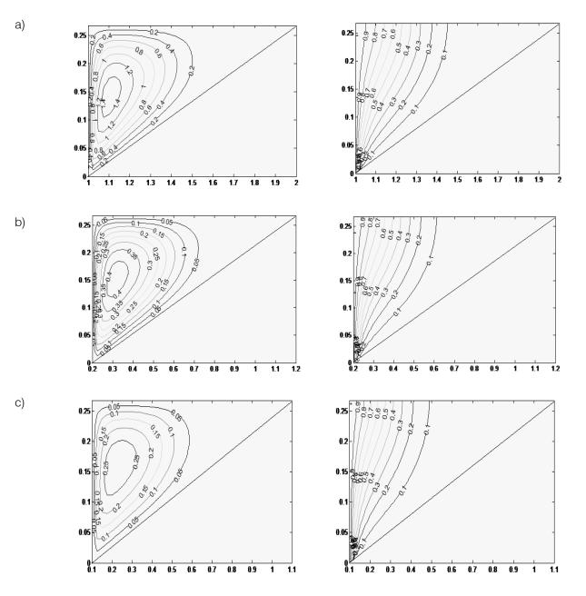
*Figure 2*: Streamlines (left) and Isotherms (Right) for Ra=100,  $C_A = 75$ ,  $\epsilon = 0.01 R_r = 1 b$ )  $R_r = 5 c$ )  $R_r = 10 a$ )
