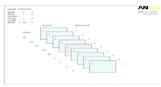
Figure 2: Layer stacking sequence of composite pressure vessel [±45/0] FW
