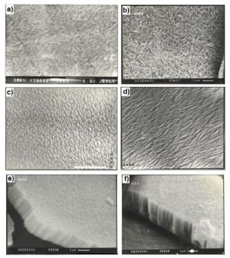
*Figure 2*: Microgfotoraphs of the surface of (a-d) and cleavages (e, f) coating  $MoS_2$  (a, c, e) and  $WSe_2$  (b, d, f), applied at a temperature of 523 K ( $MoS_2$ ) to 653 K ( $WSe_2$ ) at location samples in the center of the plate (a, b, e, f) and on its periphery (c, d)
