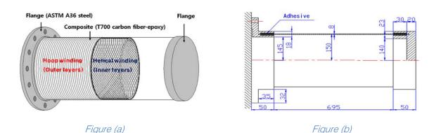
Figure 1: (a) Schematic of a filament-wound composite cylinder with flange (b) Dimension of the cylinder
