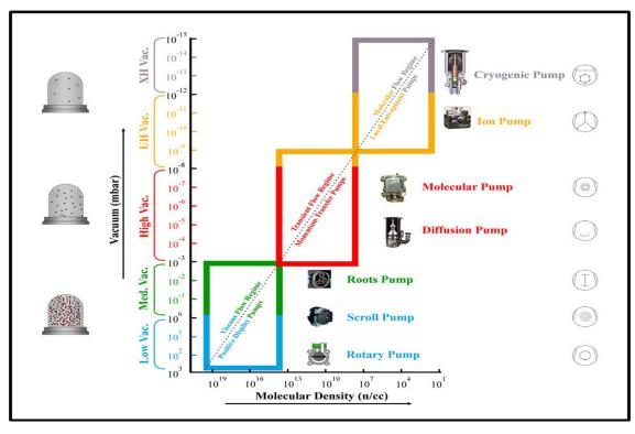
Figure 3: Pump classification on the basis of degree of vacuum and molecular density [3]
