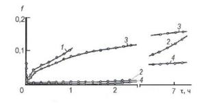
*Figure 6* : Dependence of the friction coefficient on the duration of the test coatings: 1 -  $MoS_2$ ; 2 -  $MoS_2$ Д<sub>x</sub>; 3 -  $(Mo_2N-M_kN_mX_n - MoS_2)$ ; 4 -  $(Mo_2N-M_kN_mX_n - MoS_2$ Д<sub>x</sub>)
