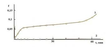
*Figure 5*: Coefficient of friction on the duration of the test coatings doped  $MoS_2$  (1 -  $MoS_2$ ; 2 -  $MoS_2D_x$ )
