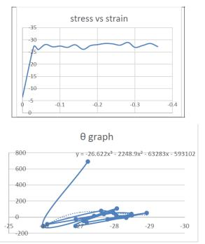
*Figure 6 :* Strain hardening curve along with stress strain curve at 350°c
