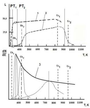
*Figure 9*: Dependence characteristics L (a) and the particle energy distribution (b) of temperature
