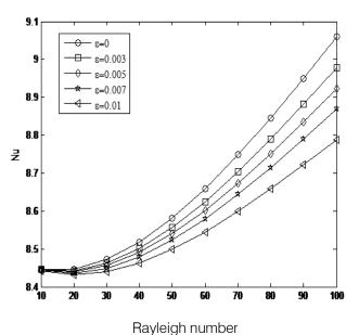
Figure 7:  $\overline{Nu}$  variations with Ra at hot surface for different values of  $\varepsilon$  at C<sub>A</sub> = 75, R<sub>r</sub>=1
