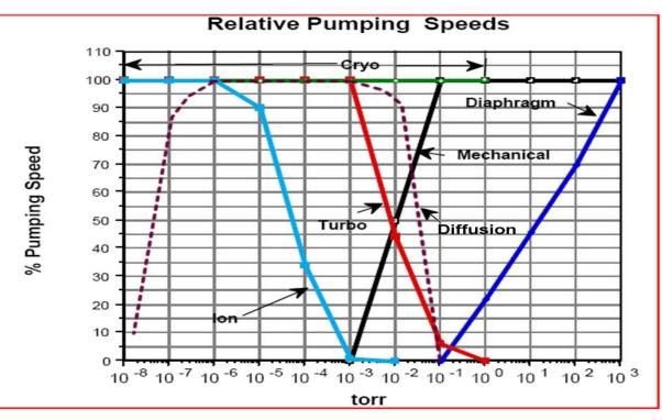
Figure 10: The change of relative pumping speed with pressure of some common vacuum pumps [7]
