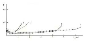
*Figure 8*: Dependence of the friction coefficient on the duration of the test doped coatings WS<sub>2</sub> and WSe<sub>2</sub> with wear sublayer Cr<sub>2</sub>O<sub>3</sub>, deposited on titanium alloys: (1-WS<sub>2</sub>; 2-WSe<sub>2</sub>; 3-WSe<sub>2</sub>Ga<sub>x</sub>; 4-WS<sub>2</sub>Ga<sub>x</sub>)
