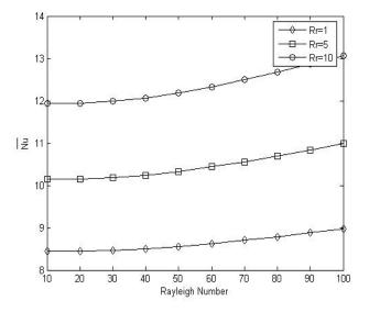
Figure 6 : Nu variations with Ra at hot surface for different values of R<sub>r</sub> at C<sub>A</sub>=75, $\epsilon$ =0.01
