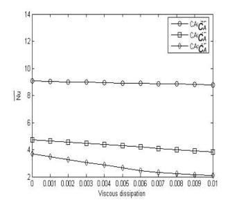
*Figure 8* :  $\overline{Nu}$  variations with  $\varepsilon$  at hot surface for different values of C<sub>A</sub> at R<sub>r</sub>=1, Ra=100
