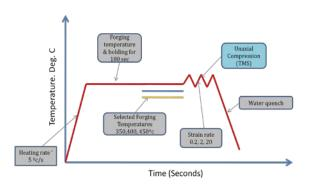
Figure 1 : Gleebel cycle for 6061 Aluminium Alloy
