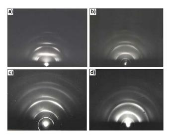
*Figure 1*: The electron diffraction patterns of coatings  $MoS_2$  (a, c) and  $WSe_2$  (b, d) a thickness of 0.5 microns, applied at a temperature 523 K ( $MoS_2$ ) and 623 K ( $WSe_2$ ), and the location of samples in the center of the plate (a, b) and at its periphery (c, d)
