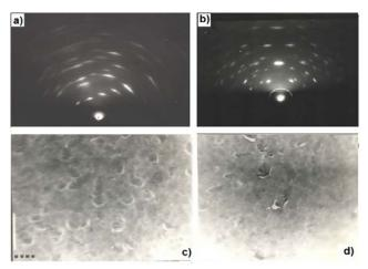
*Figure 4* : Electron diffraction (a, b) and micrographs (x5000) (c, d) coating AIN (a) and Cr<sub>2</sub>O<sub>3</sub> (b, c, d)
