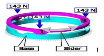
Figure 3: Sliding contact at the swiveling joint
