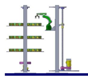
Figure 3 : Side view of the automated buffer
