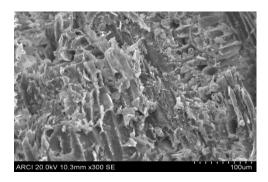
Figure 28 : Microscopic view poly acrylonitrile
