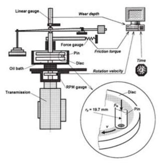
Figure 4 : Pin on disc setup
