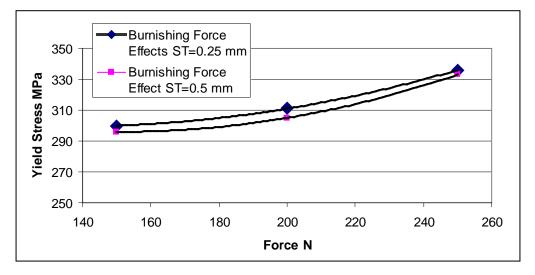
Figure 7: (b) The effect of burnishing force on the bending stress at high table speed
