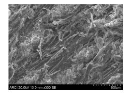
*Figure 29 :* Microscopic view poly acrylonitrile affinity of 6M concentration treated neem wood
