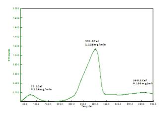
Figure 24 : DTG curve for Acrylonitrile of 6M concentrated treated cork wood
