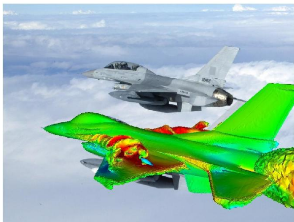
Figure 2 : Visualization of vortex flow past an aircraft
