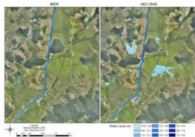
Figure 10 : 10 years RT flood: Areas subject to flooding
