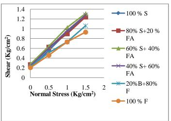
*Fig. 6 :* Direct shear test of Fly Ash and Sand Mixtures in Wet Condition
