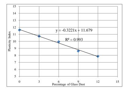
Figure 4 : Variation of Plasticity Index with Percentage of Glass Dust
