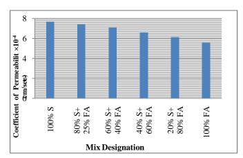
Fig. 4 : Coefficient of permeability of Fly Ash and Sand mixtures
