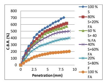
*Fig. 8 :* CBR value of Fly Ash and Sand Mixtures in Soaked Condition
