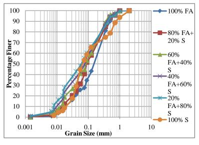
Fig. 1 : Grain Size distribution curve of Fly Ash and Sand mixtures
