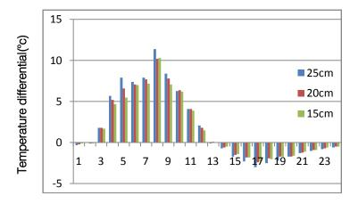
*Figure VIII :* Actual Temperature Differential at edge of PQC Slabs
