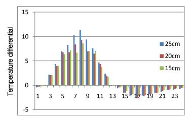
Figure 11 : Actual Temperature Differential at edge of HVMPC Slabs
