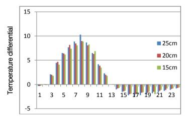
Figure 13 : Actual Temperature Differential at corner of HVFAC Slabs
