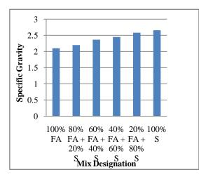
Fig. 2 : Specific gravity of fly ash and Sand mixtures
