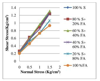
*Fig. 5 :* Direct shear test of Fly Ash and Sand Mixtures in Dry Condition
