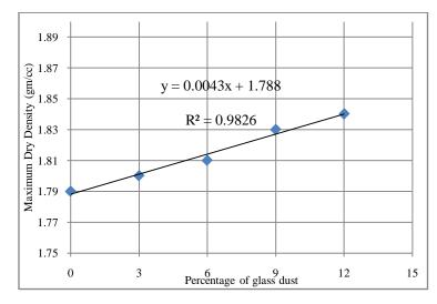
Figure 2 : Variation of Maximum Dry Density with Percentage of Glass Dust
