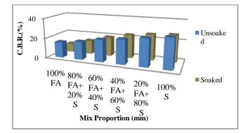
*Fig. 9*: CBR value of mixtures of Fly Ash and Sand in soaked and Unsoaked Condition
