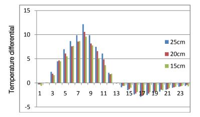
Figure 8 : Actual Temperature Differential at middle of HVMPC Slabs
