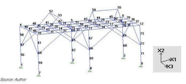
Fig. 2 : Indication of the structure nodes
