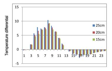
Figure 12 : Actual Temperature Differential at corner of PQC Slabs
