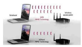
Fig. 1: MIMO technology uses multiple radios to transfer more data at the same time
