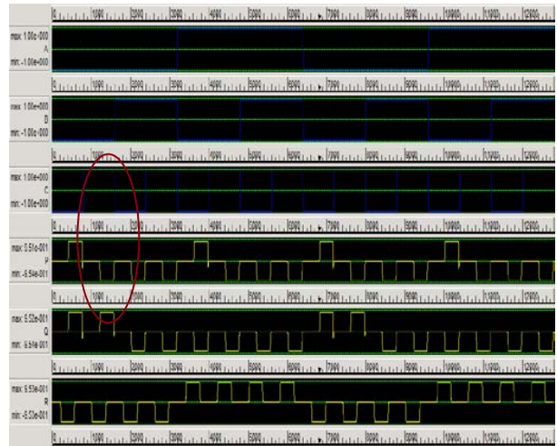
Figure 7 : Simulated input output waveforms of MCL gate with 0.5 clock cycle delay
