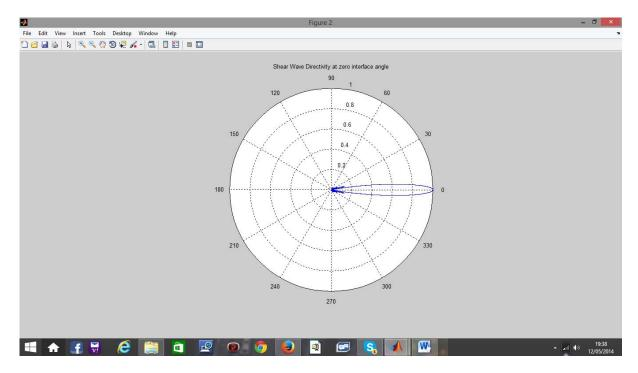
Fig. 6 : Directivity pattern of shear wave in Steel/Rexolite at 0º interface angle
