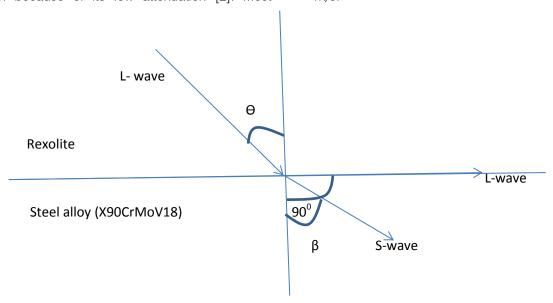
Fig. 1 : Refraction of shear waves into the sample
