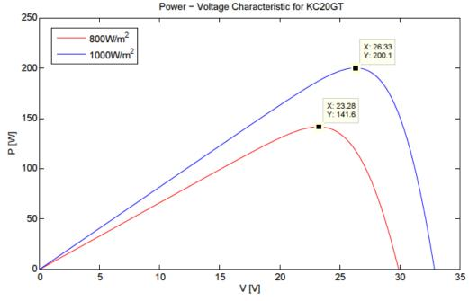
Figure 8e : Power-voltage characteristics of KC200GT, [12]
