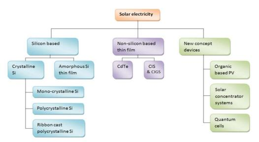
Figure 10a : PV cells material Technology [13]
