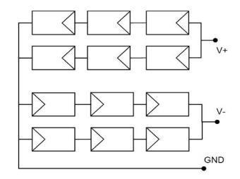
*Figure 7f :* Modules forming a panel connected in series-parallel with center grounded to provide + and – supplies (fuses and diodes not shown), [10]
