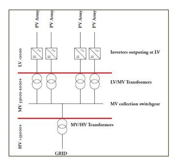
Figure 9: Typical Transformer Locations and Voltage Levels in a Solar Plant where Export to Grid is at HV, [1]
