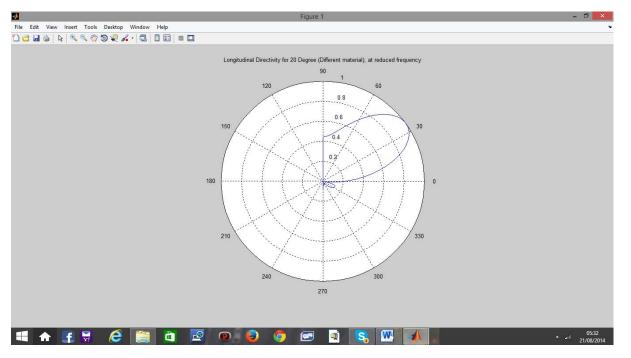
Fig. 11 : Directivity pattern of longitudinal wave in Steel/Rexolite at 20º angle and 0.5MHz
