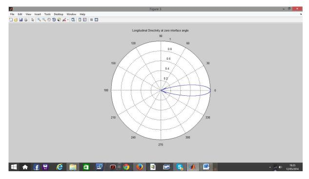
Fig. 5: Directivity pattern of longitudinal wave in Steel/Rexolite at 0° interface angle
