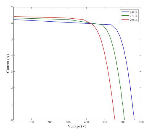
Figure 8d : The effect of temperature on the I-V characteristics for typical module at 800 W/m<sup>2</sup> irradiance, [11]
