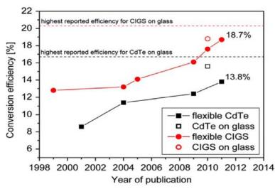
*Figure 10c*: Conversion efficiencies of flexible CdTe and CIGS solar cells fabricated by low temperature processes Also shown is the in-house reference on glass and the highest reported efficiency for each technology, [13]
