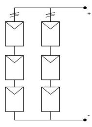
*Figure 7e :* Modules forming a panel connected in series-parallel with internal by pass diodes and series fuses, [10]
