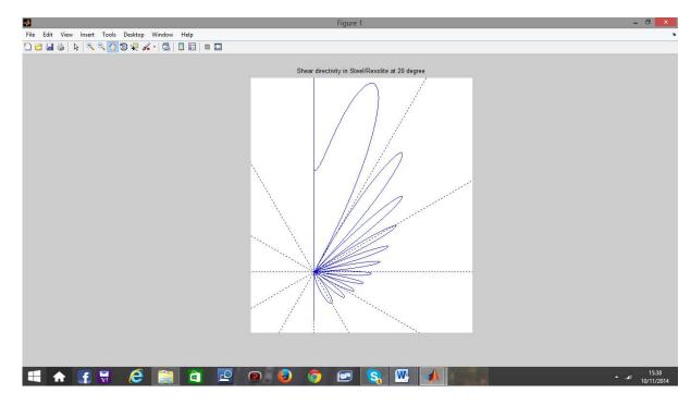
Fig. 9 : Directivity pattern of shear wave in Steel/Rexolite at 20º interface angle, 1MHz
