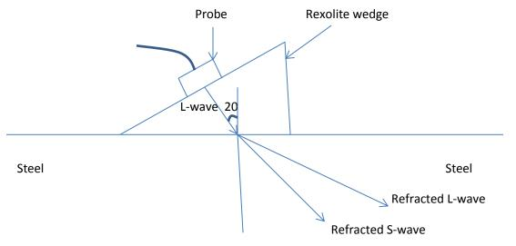
*Fig. 7 :* Ray propagation through 20<sup>o</sup> Rexolite wedge into Steel
