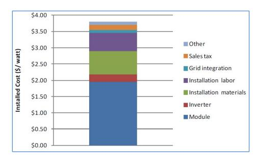
Figure 6b : Utility-scale PV facility by cost component, 2011, [7]
