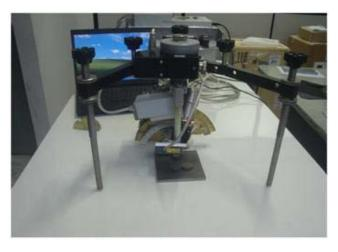
Figure 2 : Portable diffractometer used in the analysis of residual stresses
