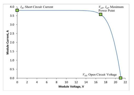
Figure 8a : Photovoltaic module I-V characteristics
