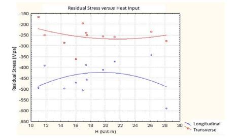
*Figure 10 :* Influence of heat input on the level of longitudinal and transverse residual stresses, and the interaction between the stress levels in the FCAW process
