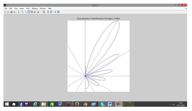
Fig. 12: Directivity pattern of shear wave in Steel/Rexolite at 20<sup>o</sup> angle and 0.5MHz
