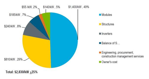
Figure 6a : Utility-scale PV facility by cost component, [7]
