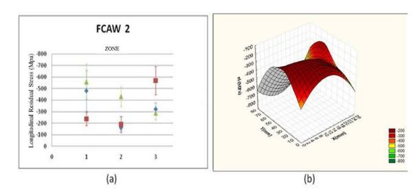
*Figure 6 :* Mean values of longitudinal residual stresses and their respective uncertainties (a); Field of longitudinal residual stresses into the coating -2(b)
