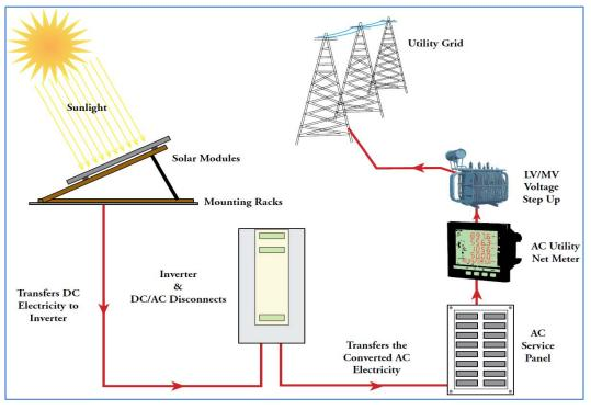
Figure 1 : Overview of Solar PV Power Plant, [1]
