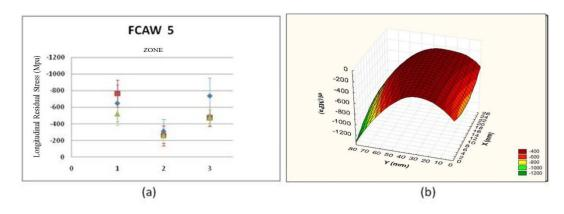
*Figure 8 :* Mean values of longitudinal residual stresses and their respective uncertainties (a); Field of longitudinal residual stresses into the coating - 5 (b)
