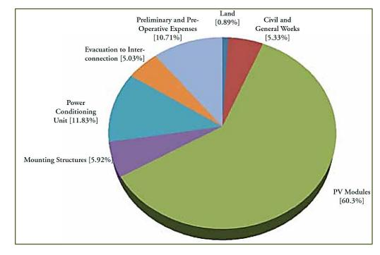
*Figure 18 :* Cost breakdown of PV power station, [21]
