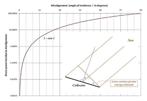
*Figure 15 :* The effective collection area of a flat-panel solar collector varies with the cosine of the misalignment of the panel with the Sun, [21]
