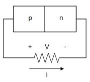
Figure 7c : Operating scheme of photovoltaic cell, [10]
