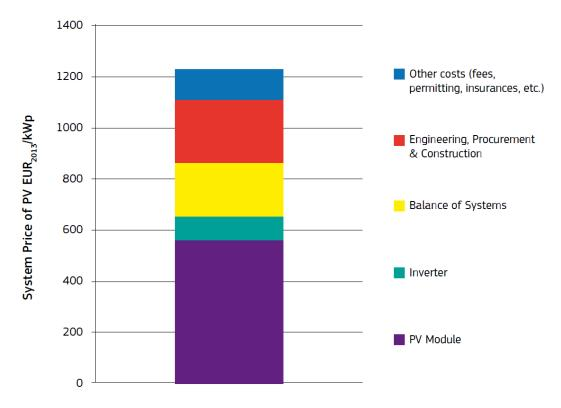
Figure 6c : Utility-scale PV facility by cost component, 2013, [3]
