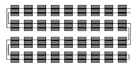
Figure 7d : Sturcture of a PV module consisting of 36 cells connected in series, [10]
