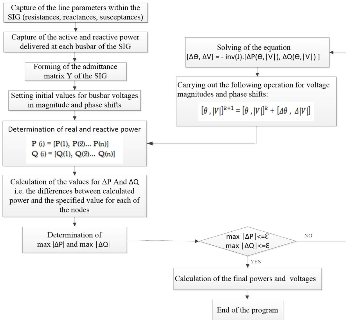
Figure 1 : Flow chart of the Newton-Raphson's method[8, 7]
