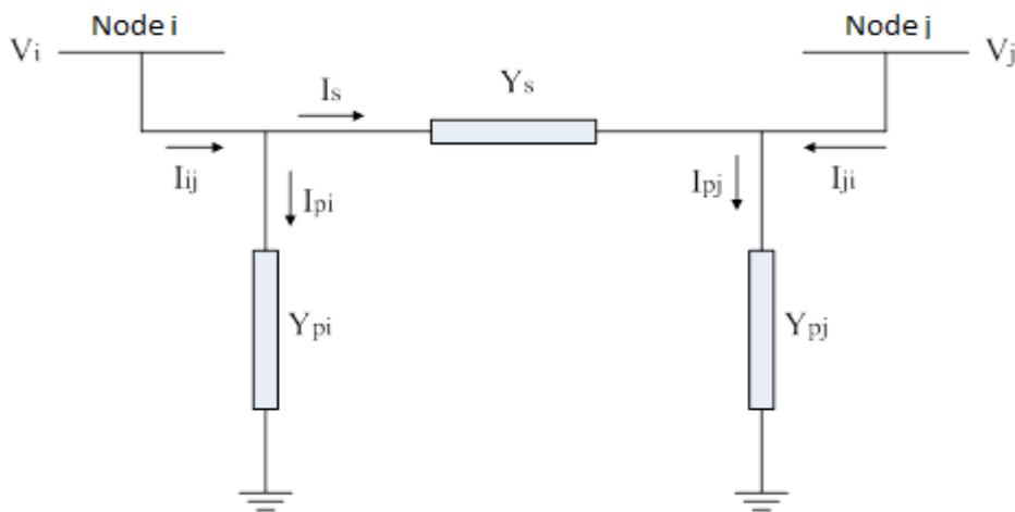
Figure 2 :  $\pi$ -Model of the transmission line [1]
