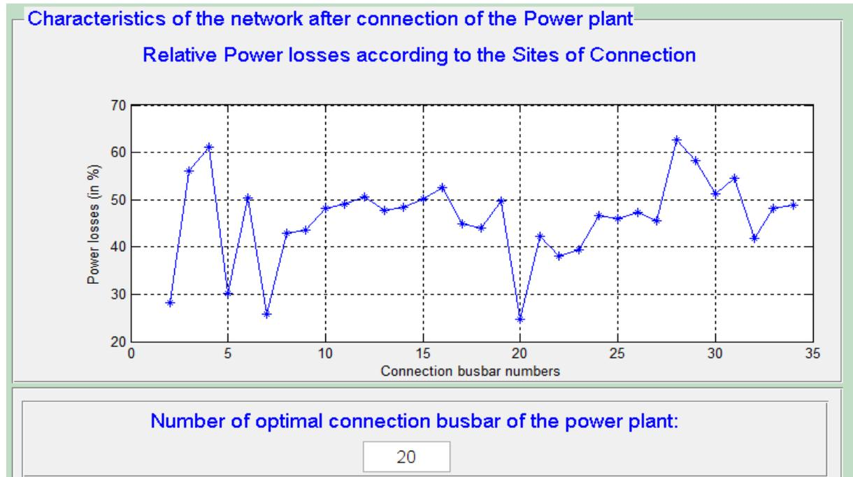
Figure 7: Results obtained after successively connecting Kribi to all the busbars of the SIG
