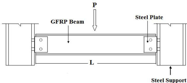
Fig. 1 : Schematic of I-Section GFRP beam
