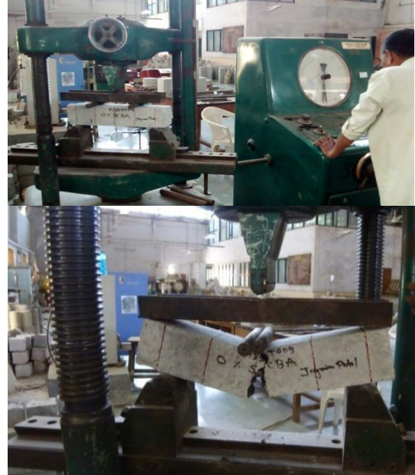
Figure 6 : Testing of beam for flexural strength and sample after testing
