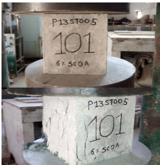
Figure 5 : Compression testing of concrete cubes specimen before and after testing
