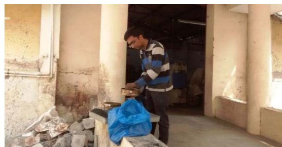
Figure 3 : Checking Sugar cane bagasse ash taken from sugar mill and removing unburned particles
