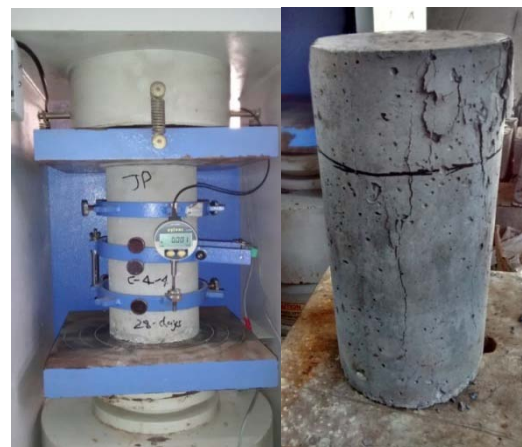
Figure 7 : Testing of modulus of elasticity of concrete cylinder and sample after testing
