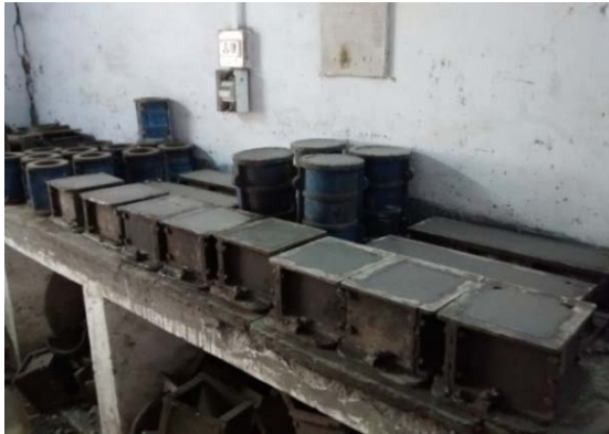
Figure 4 : Specimen after casting putting for dry for 24 hours
