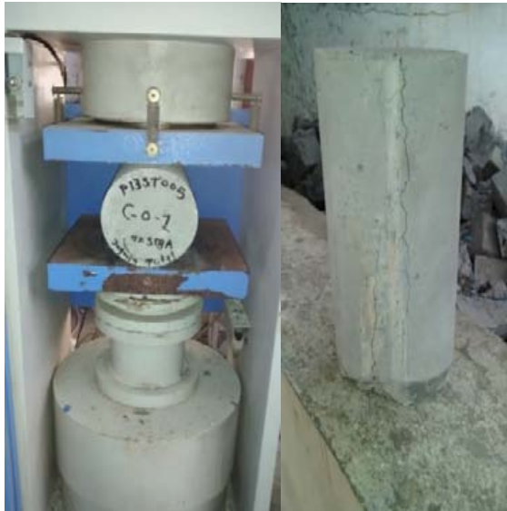
Figure 8 : Split tensile testing of concrete cylinder and sample after testing
