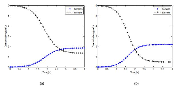
Fig. 1: Unsteady state concentration of biomass and substrate at Si=6 for :(a)D=0.3, (b) D=0.8
