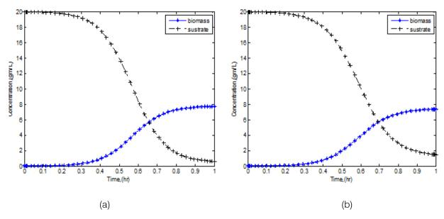
Fig. 2: Unsteady state concentration of biomass and substrate at Si=20 for ;(a) D=0.3, (b) D=0.8
