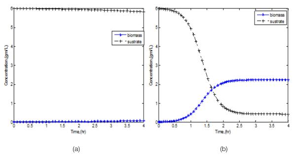
Fig. 7: Effect of pH on the process at D=0.3 and Si=6 for; (a) pH=2, (b) pH=4.
