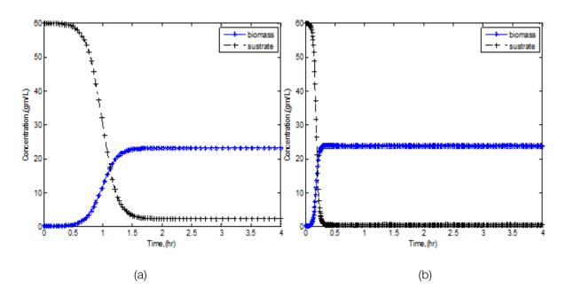
Fig. 8: Effect of pH on the process at D=0.3 and Si=60 for; (a) pH=2, (b) pH=4
