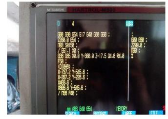
Figure 23 : G-code for Drilling
