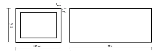
Figure 16 : Rectangular Cross Section of duct
