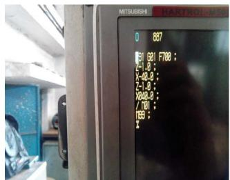
*Figure 25 :* G-code for Milling
