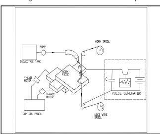
*Figure1* : Wire electrical discharge machining Process
