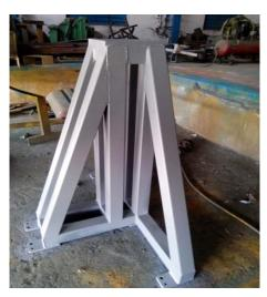
Figure 9 : Motor mounting
