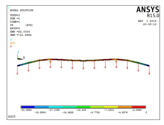
Figure 20 : Deformed Duct
