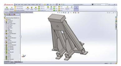
Figure 8 : CAD Model of Motor mounting
