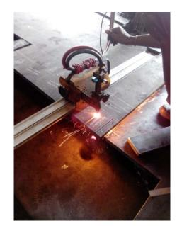
Figure 21 : Gas Cutting Process
