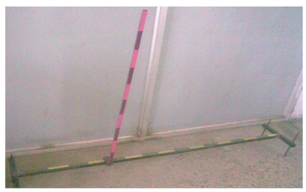
Figure 2 : Linear scales for measurement of parabolic profil
