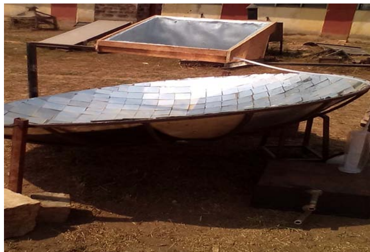
Figure 2 : Pictorial view of the parabolic reflector dish coupled single slope basin solar still
