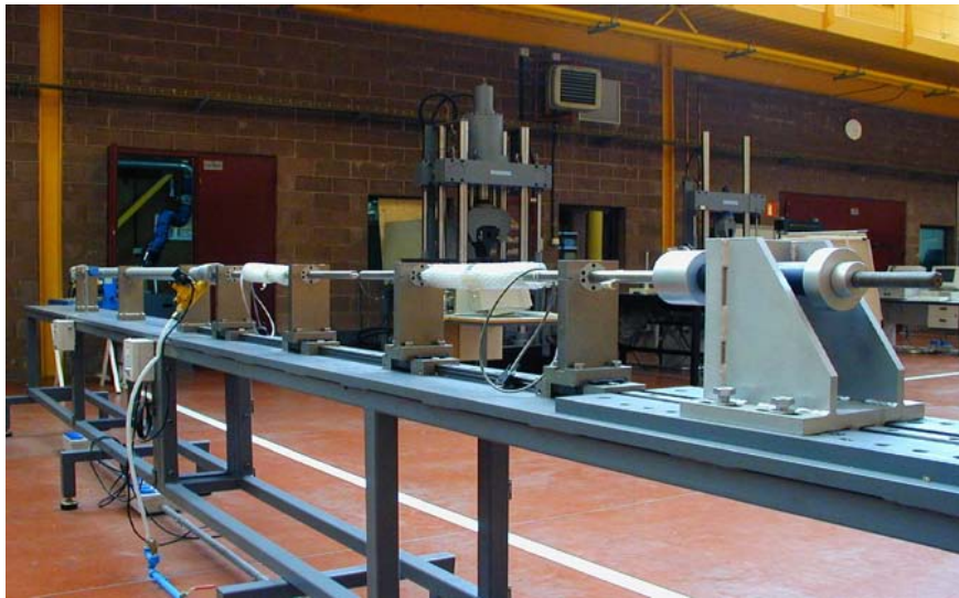
Figure 1: Split Hopkinson Tension Bar apparatus as installed in the Universidad Carlos III de Madrid Engineering Laboratory.
