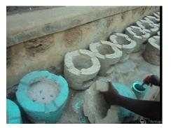
*Pictures 2 :* volcanic stoves (RONDEREZA URUTARE) in the painting process at Muneza Biomass Engineering Company site
